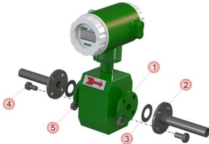
Fig.2.3 - Installation of EMIS-MAG 270 in the pipeline
