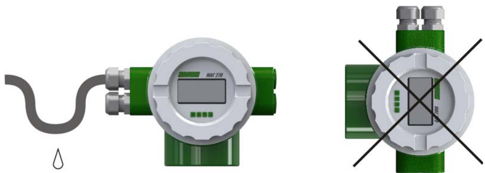
Fig.2.8 - Cables and cable glands arrangement
