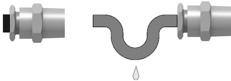
Fig.2.13 U-shaped cable loop
